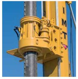
The standard Kelly bar is 4/45, The 3/35, 4/50, 5/64 and 6/75 types are also available. The square joint is available with sides of 150, 177, 200mm. All kelly bars have automatic blocking patented by IMT; this allows the blocking of the telescopic elements in any position, permitting the transfer of pull down, pull back and torque very quickly.
